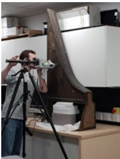
RCM0001, Conservator from the Natural History Museum using a portable device for x-ray radiography.
